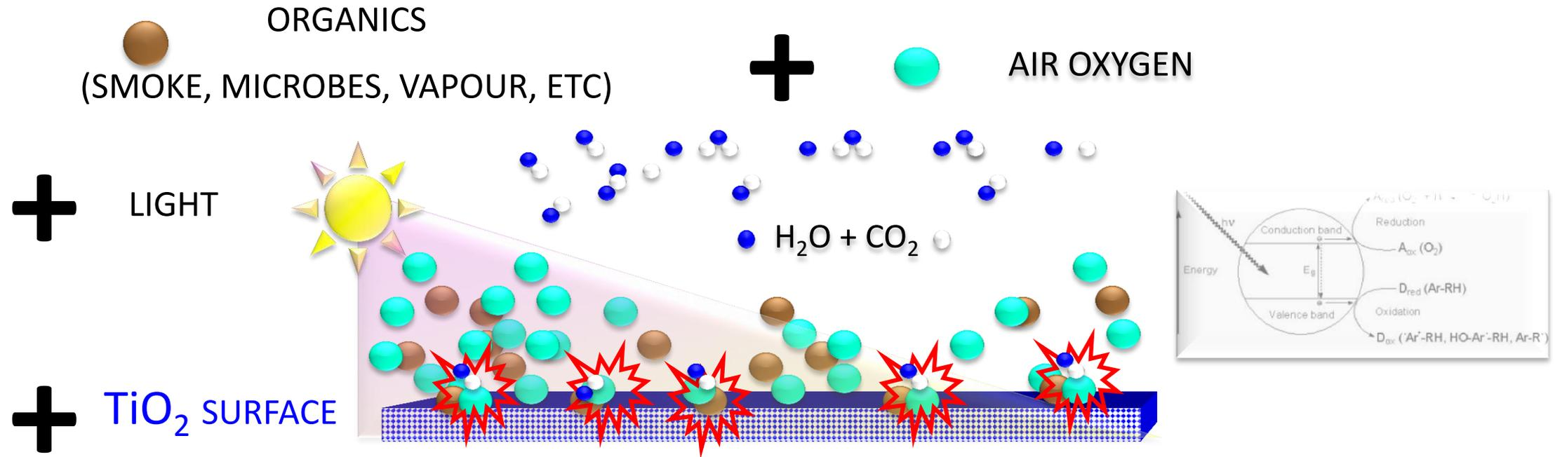
**$E_g \sim 3.2\text{eV}$  (higher oxidation potential than on chlorine, ozone or peroxide)**
